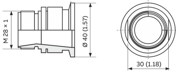
Process connection KF DN 25, to adapt inlet run and outlet run, includes 2 clamp rings and 2 sealing rings
