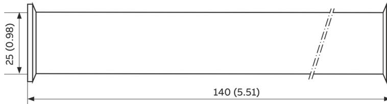
Outlet section  $5 \times D$ , both sides with KF DN 25 connection
