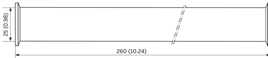
Inlet section  $10 \times D$ , both sides with KF DN 25 connection
