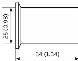
Hose adapter for KF DN 25, includes 1 small flange, as well as 1 clamping ring and 1 sealing ring each
