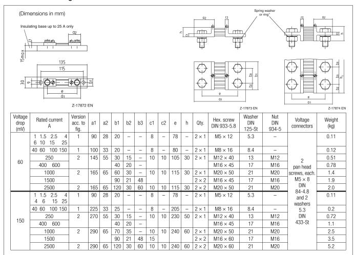
Details not provided should be selected as need be. Name of a shunt for 60 mV voltage drop and 25 A rated current: Shunt 60-25 DIN 43703
