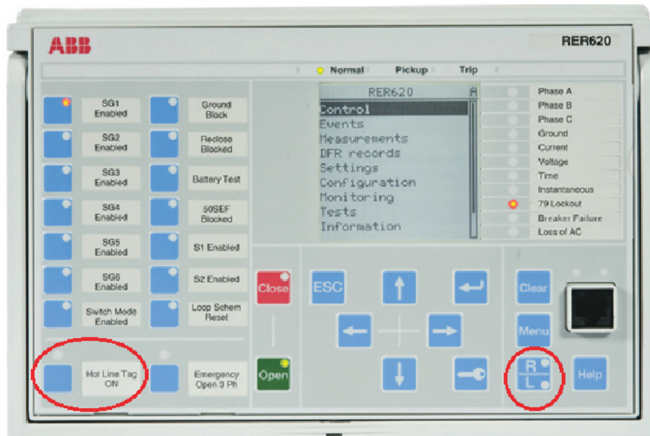
Figure 50: LHM - captioned HLT and R/L push-buttons and LEDs
