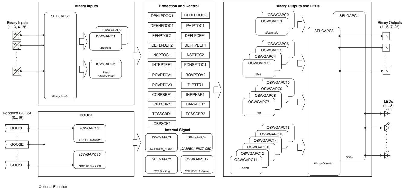
Figure 117: Configuration C switch group overview
