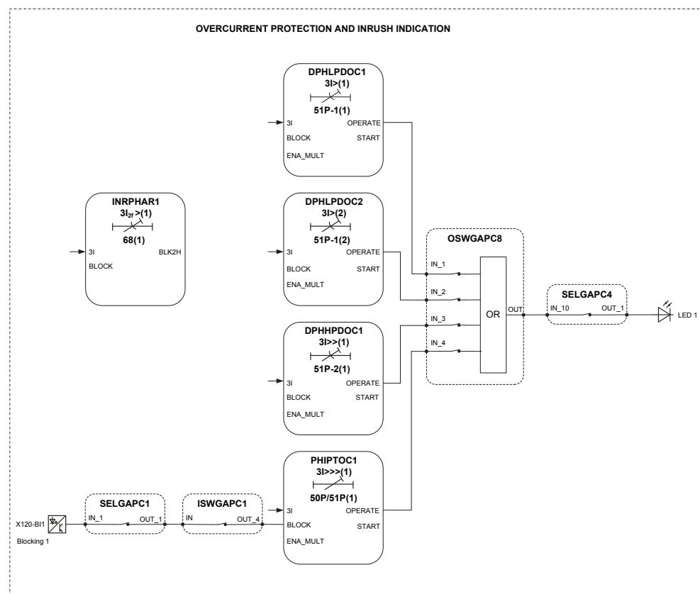
*Figure 106: Overcurrent protection*
