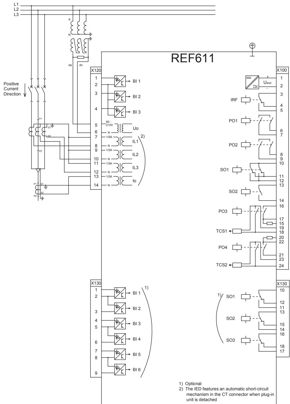
Figure 12: Connection diagram for configuration A
