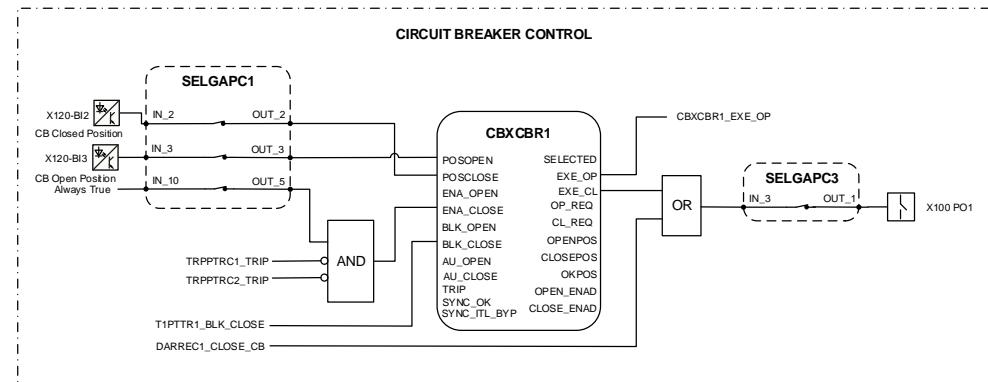
*Figure 25: Circuit breaker control*
