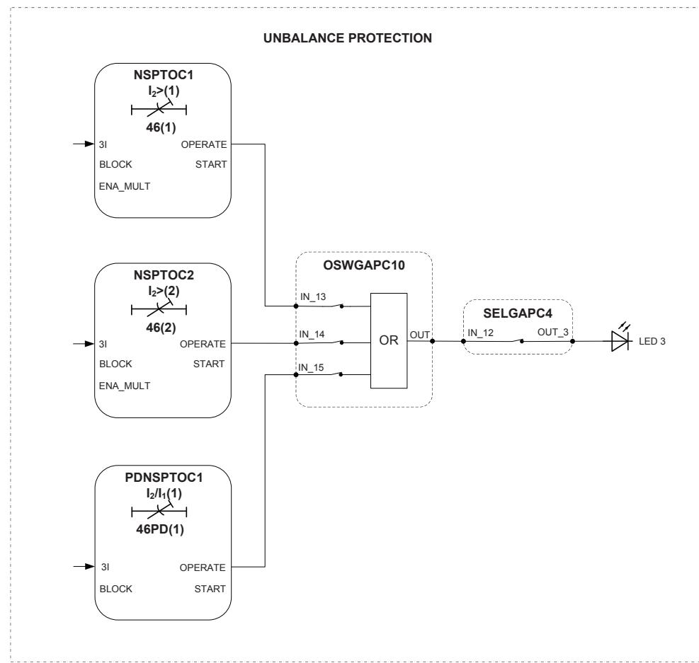
Figure 109: Unbalance protection
