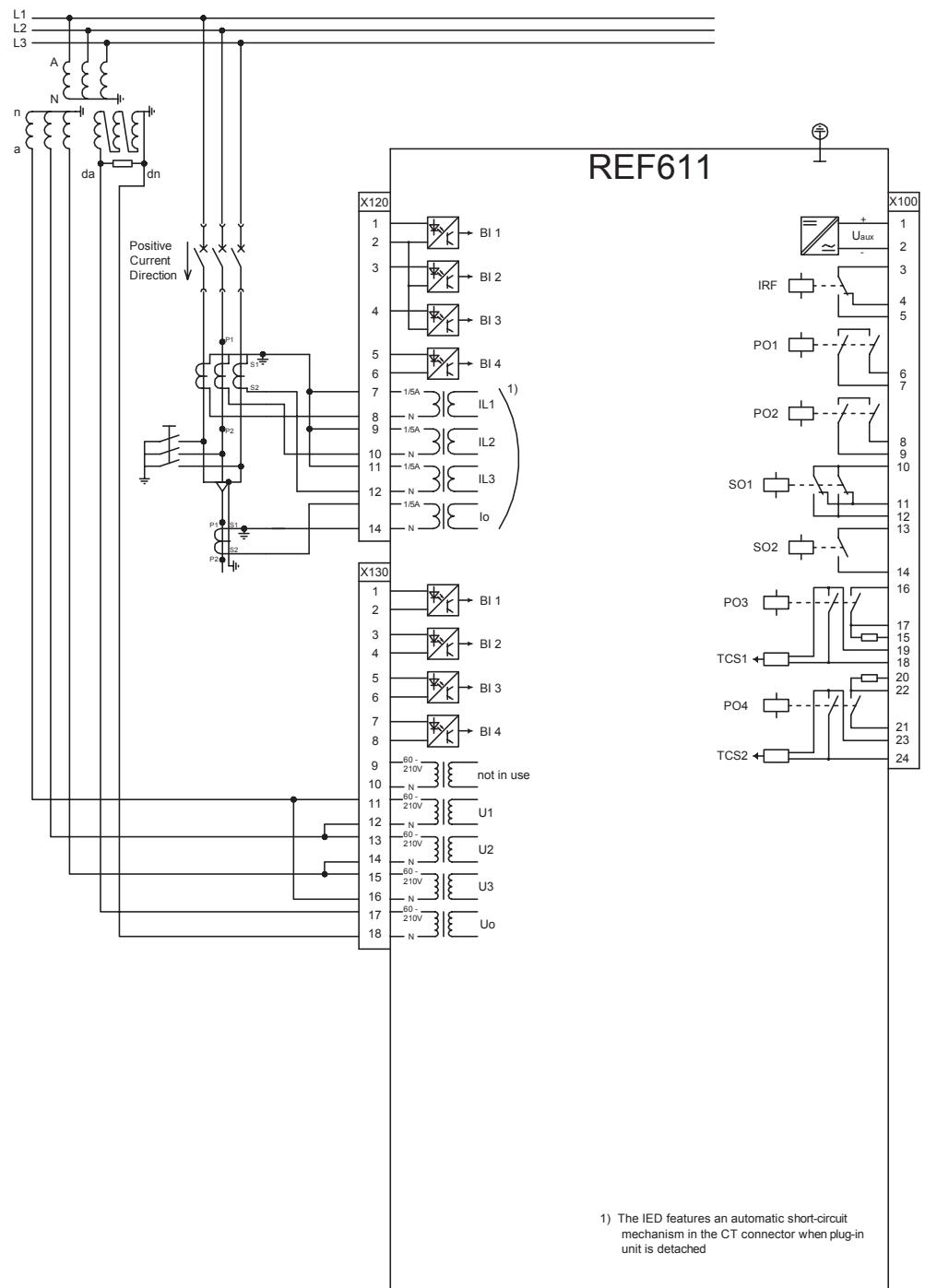
Figure 14: Connection diagram for configuration C
