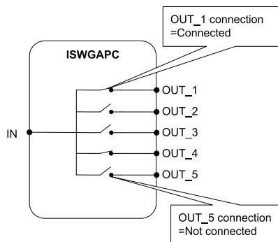
Figure 9: Input switch group ISWGAPC
