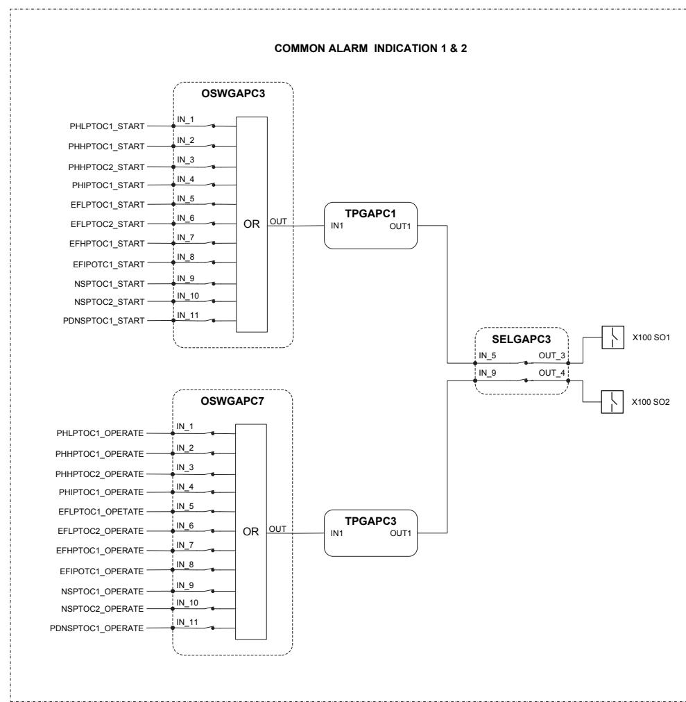
Figure 71: Common alarm indication
