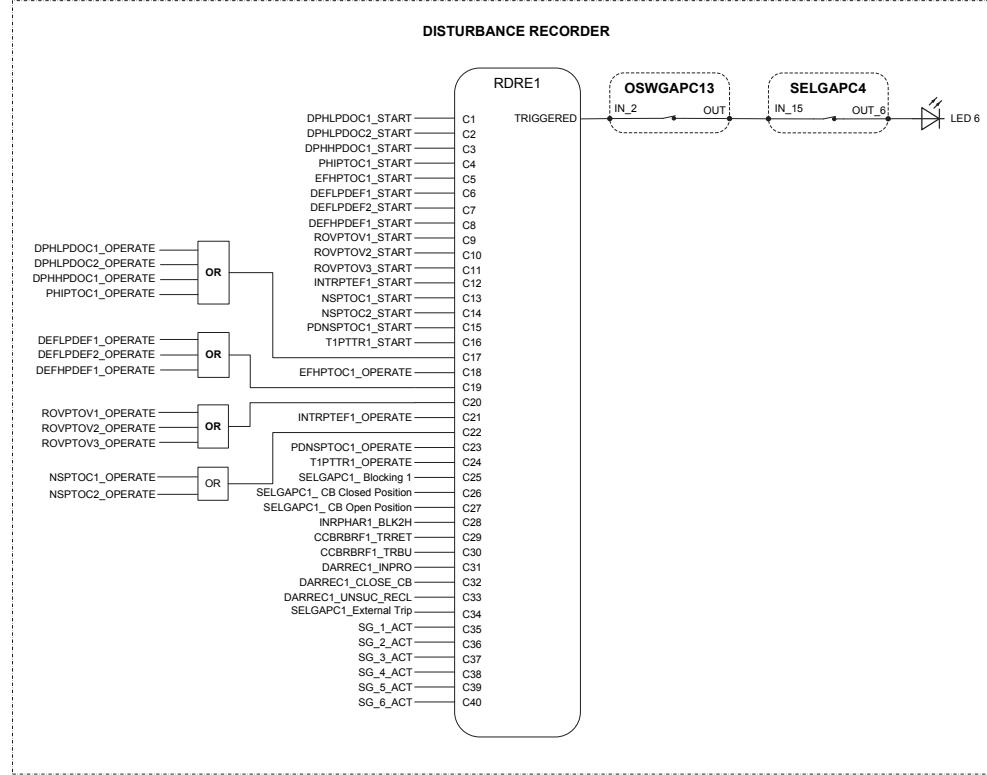
Figure 112: Disturbance recorder
