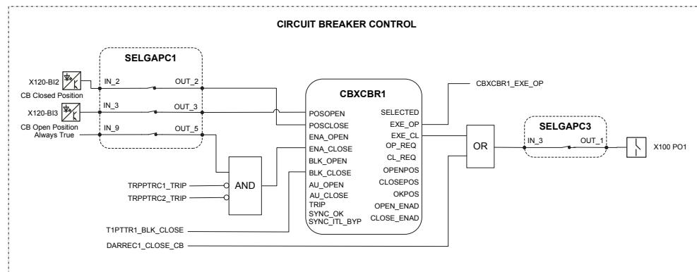
*Figure 115: Circuit breaker control*
