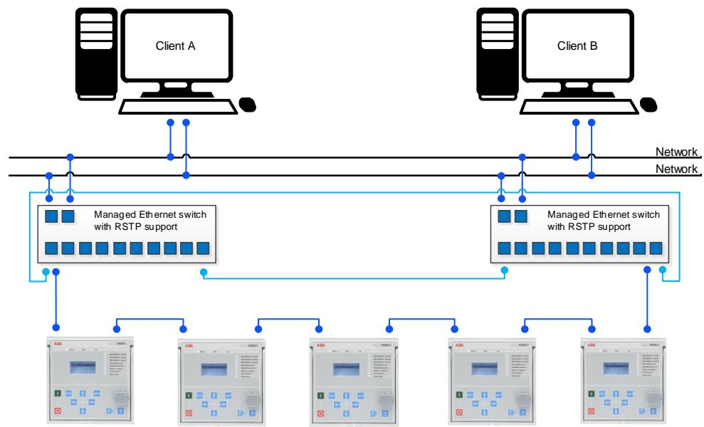
Figure 6: *Self-healing Ethernet ring solution*
