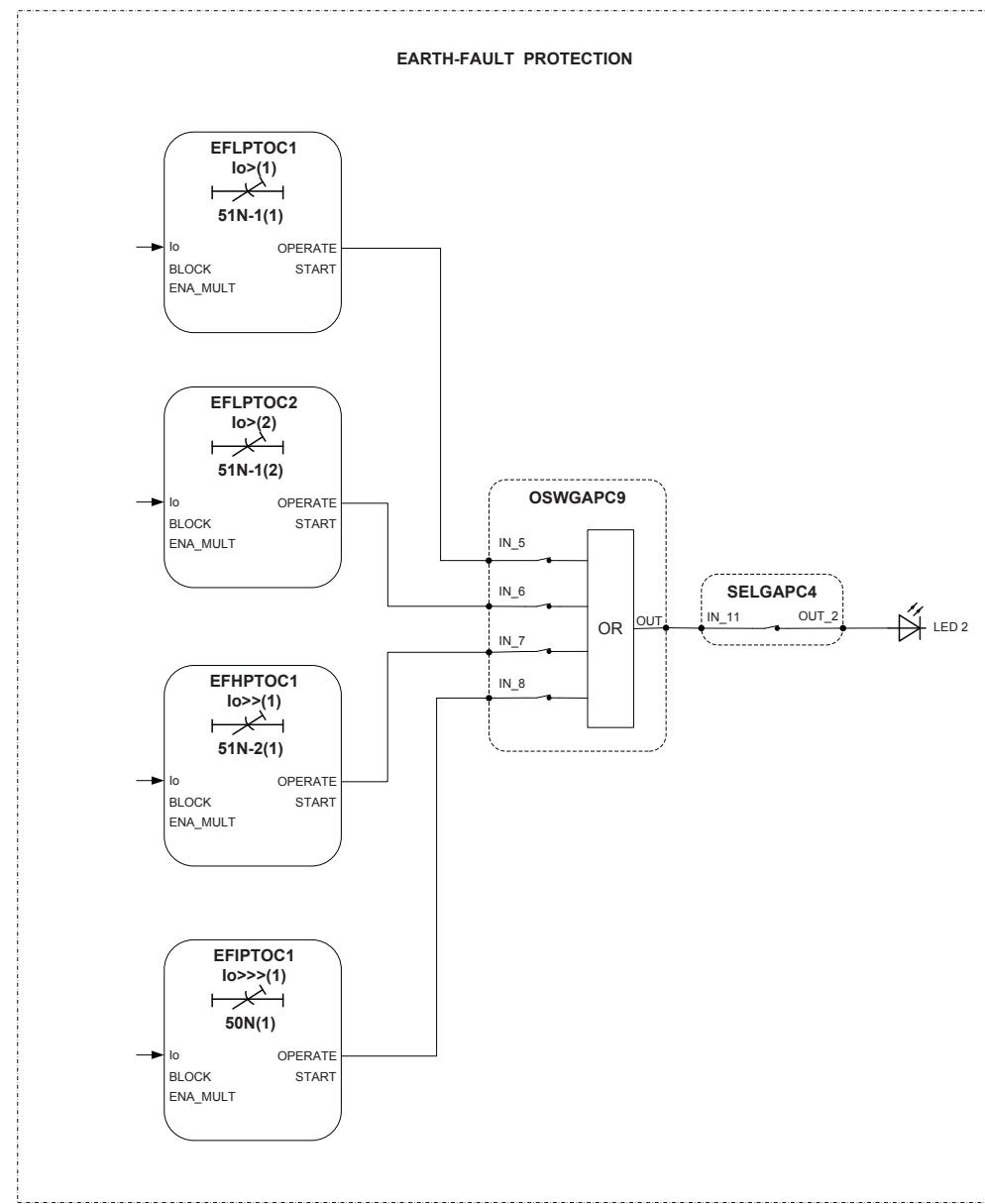
Figure 63: Earth-fault protection
