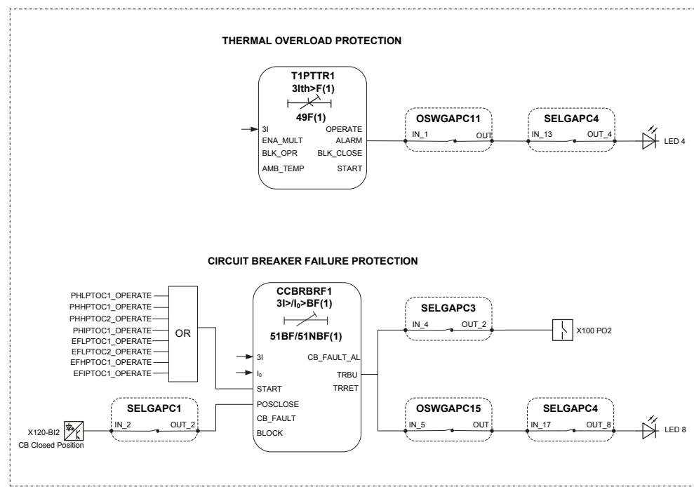
*Figure 65: Thermal overload and circuit-breaker failure protection*
