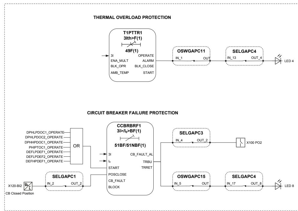
*Figure 110: Thermal overload and circuit-breaker failure protection*
