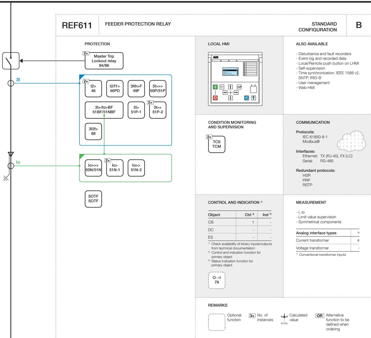
Figure 61: Functionality overview for configuration B
