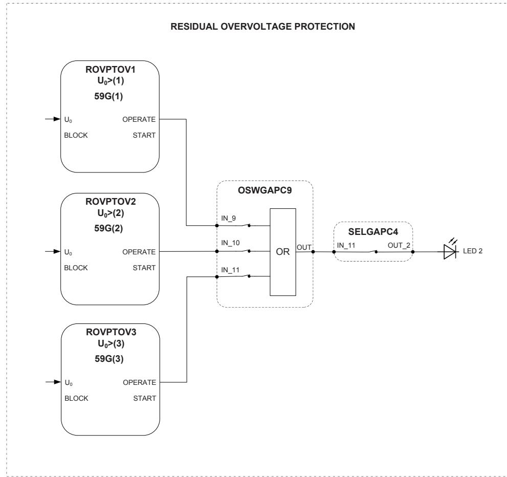
*Figure 18: Residual overvoltage protection*
