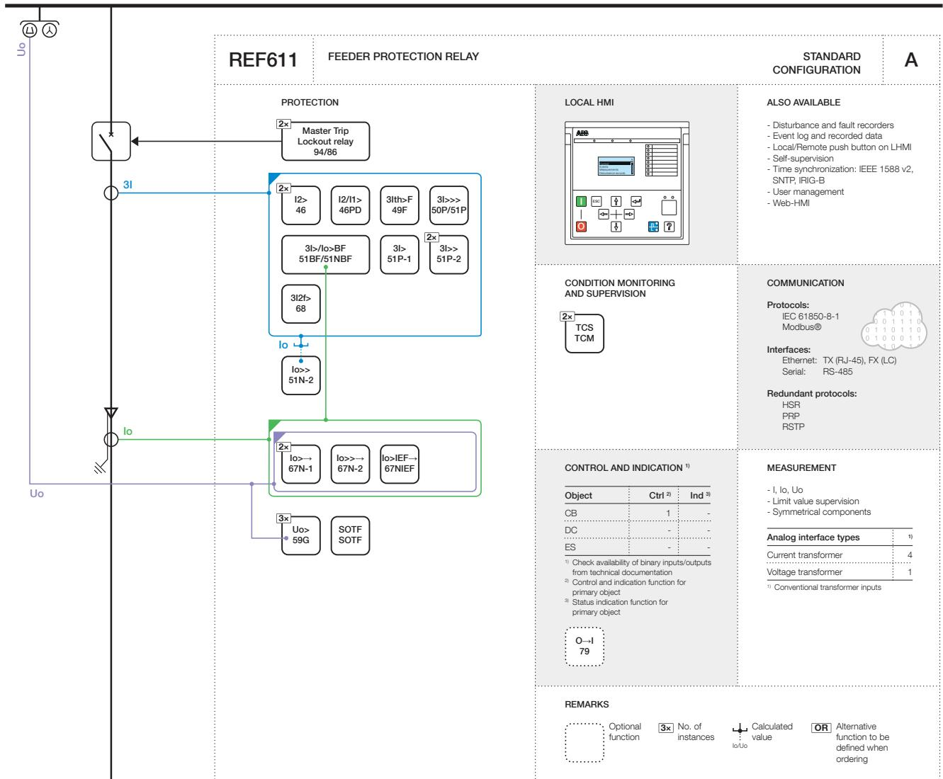
Figure 15: Functionality overview for configuration A
