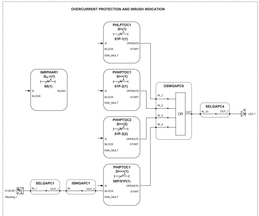
*Figure 16: Overcurrent protection*
