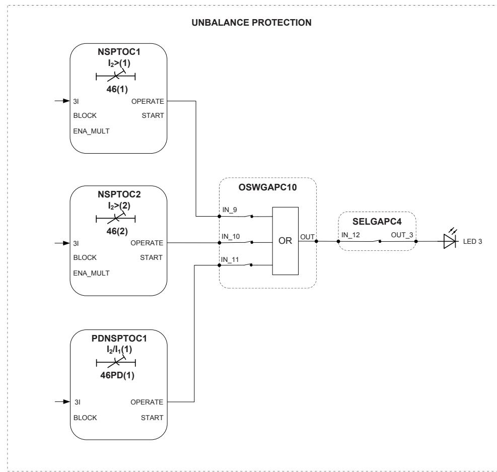
Figure 64: Unbalance protection
