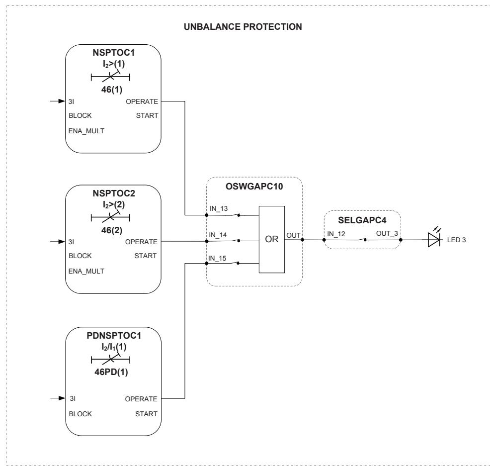
Figure 19: Unbalance protection
