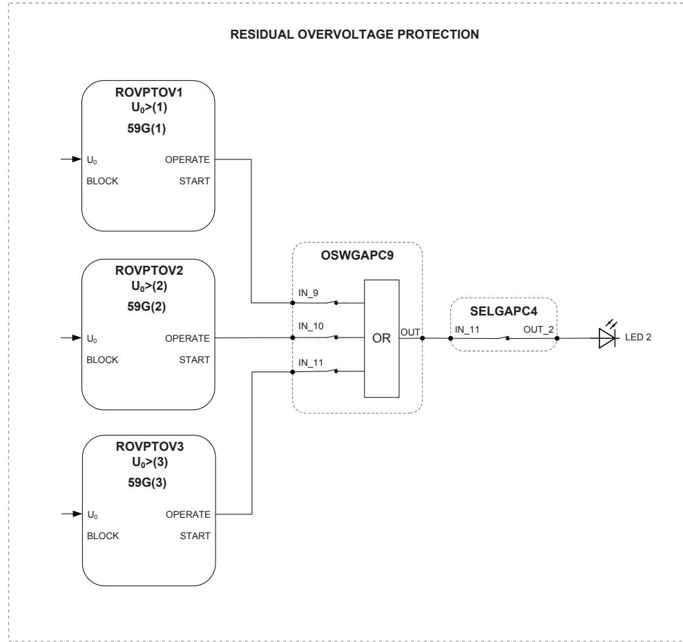
*Figure 108: Residual overvoltage protection*
