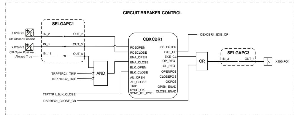
Figure 70: Circuit breaker control
