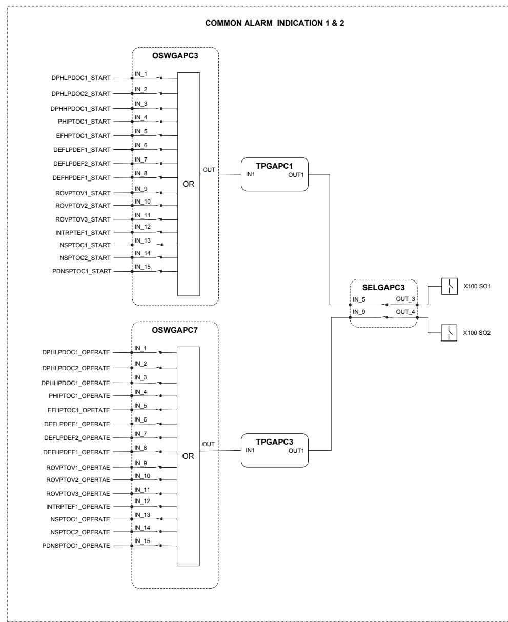
*Figure 116: Common alarm indication*
