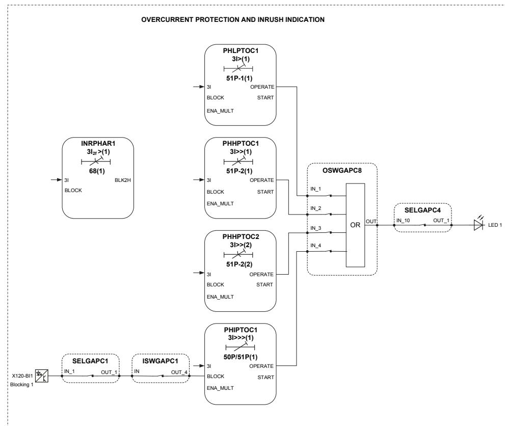
*Figure 62: Overcurrent protection*
