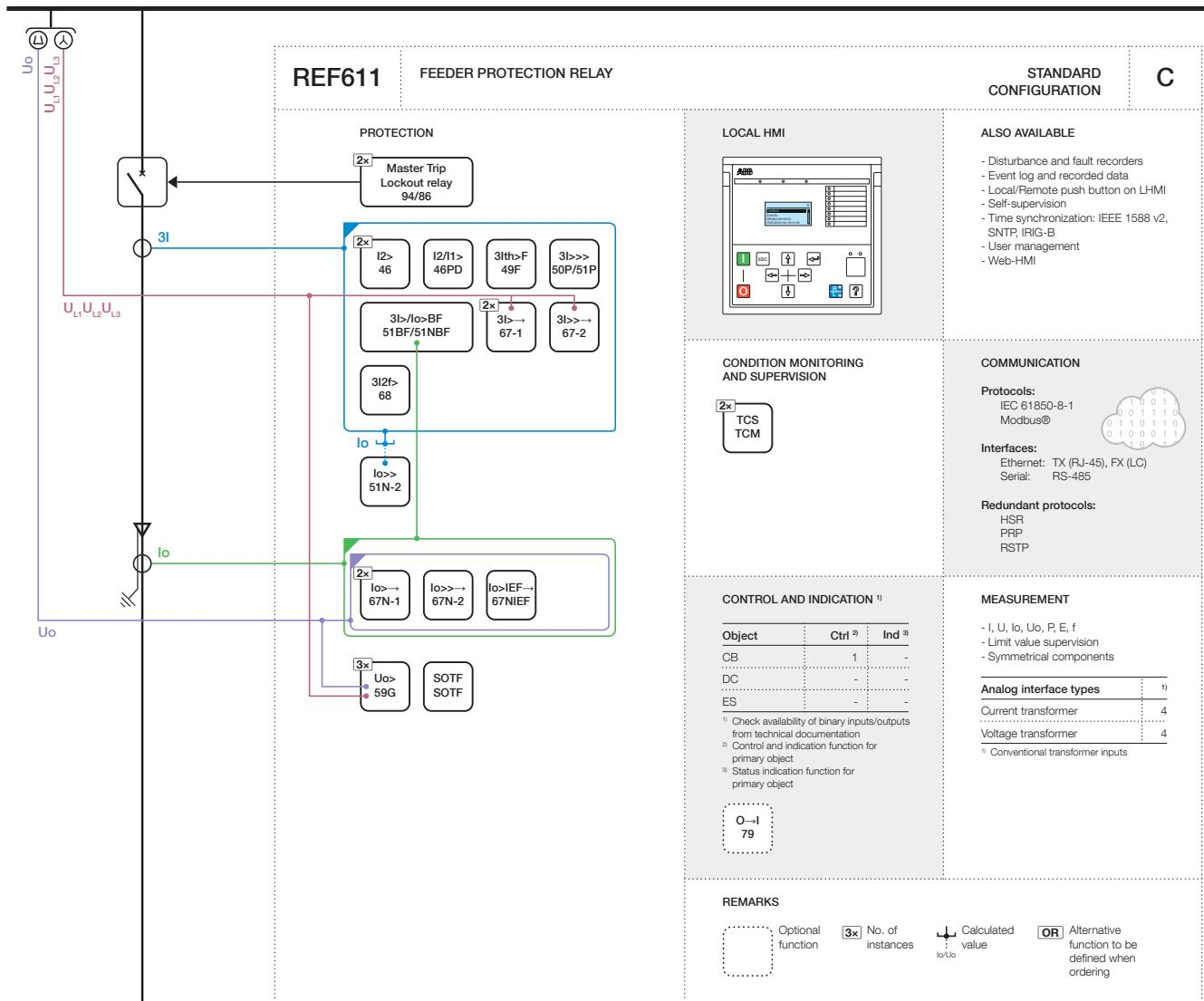
Figure 105: Functionality overview for configuration C
