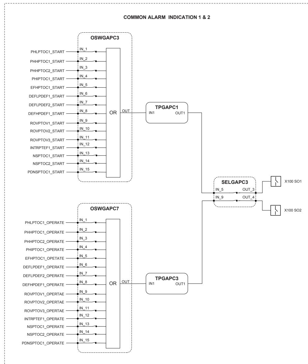
*Figure 26: Common alarm indication*
