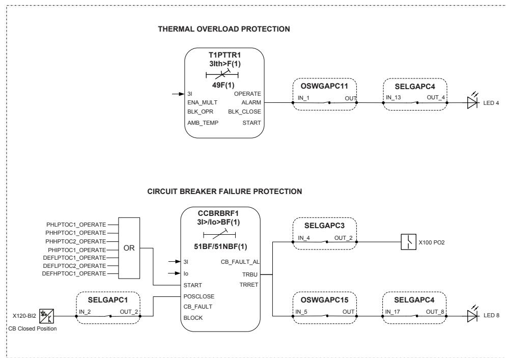
Figure 20: Thermal overload and circuit-breaker failure protection
