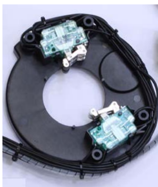
S01 and S09 micro switch on position indication disc
