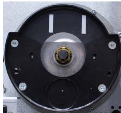
Operating bushing and front position indication disc removed.
