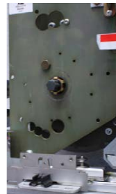
Position indication disc on 2-spring device removed.
