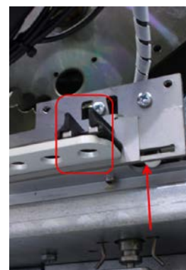
Open position of S10 micro switch
