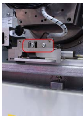
S10 micro switch installed
