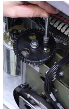
Fastening of motor from top (2 nd screw)
