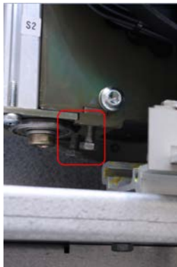
Fastening of motor from below
