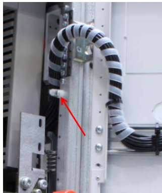
Door wiring secured with 4.2x19 torx-screw
