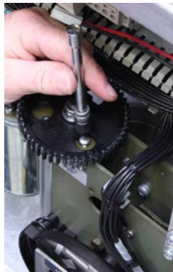
Fastening of motor from top (1 st screw)
