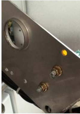
Attaching of micro switch to front plate spring device
