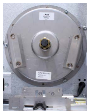
1-spring device without front plates
