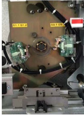
Micro switch on 2-spring device
