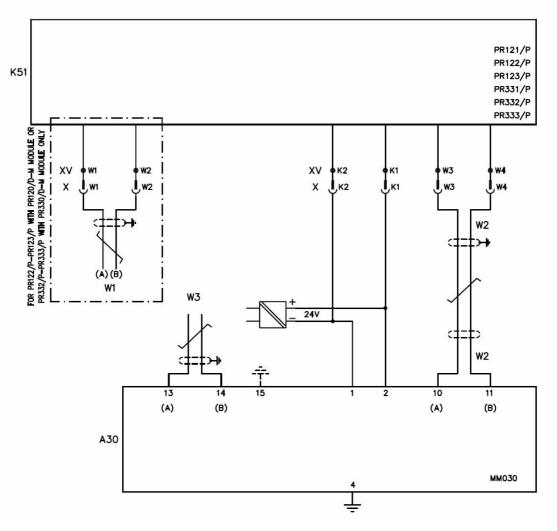
Figure 20. MM030 with PR12x/P,PR33x/P trip units circuit diagram
