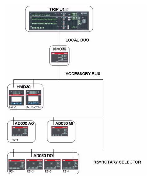
Figure 9. PR121/P and PR331/P application scenario
