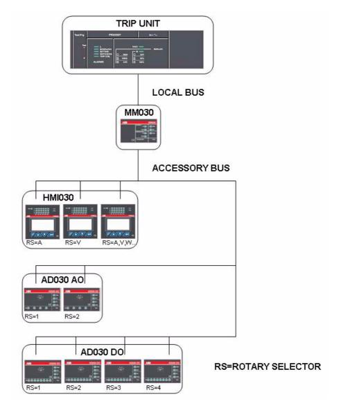
Figure 13. PR223EF application scenario
