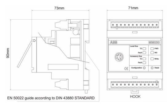
Figure 15. MM030 and Accessory Devices dimensions
