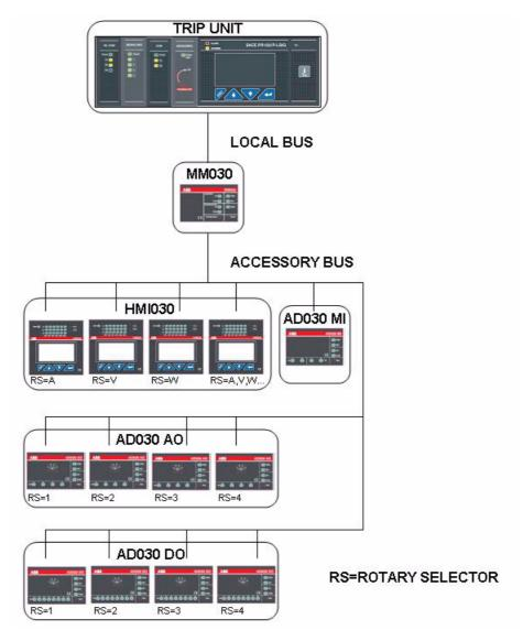
Figure 10. PR122/P, PR123/P, PR332/P and PR333/P application scenario
