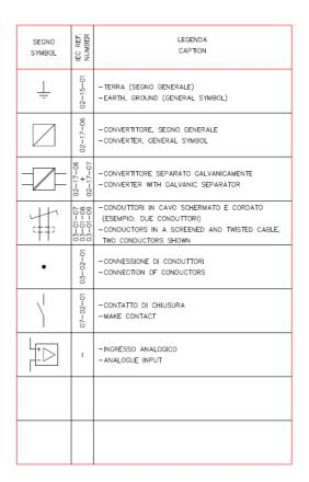
Figure 22. Graphical symbols used in circuit diagrams
