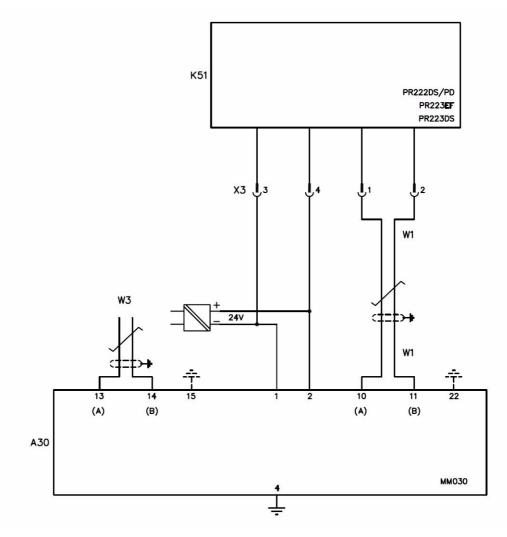
Figure 21. MM030 with PR222DS/PD and PR223 trip units circuit diagram
