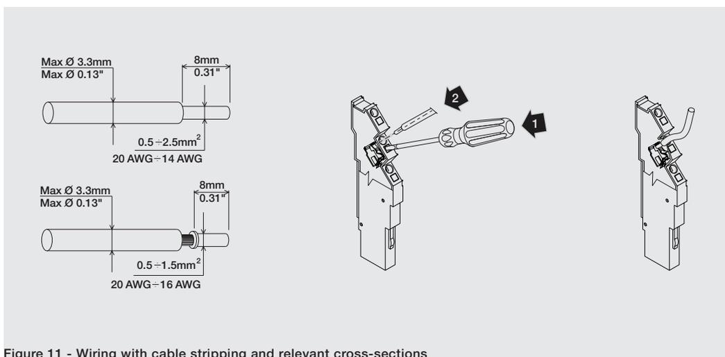
Figure 11 - Wiring with cable stripping and relevant cross-sections
