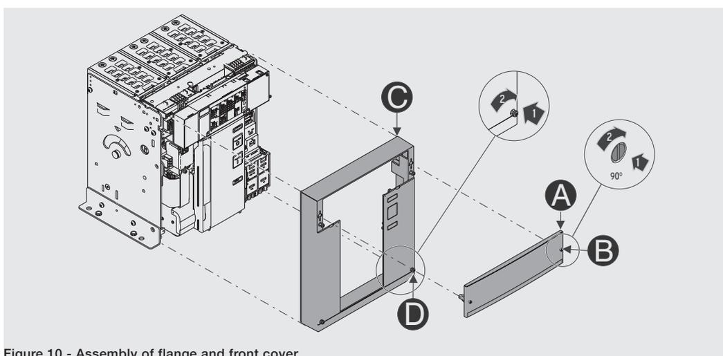
Figure 10 - Assembly of flange and front cover
