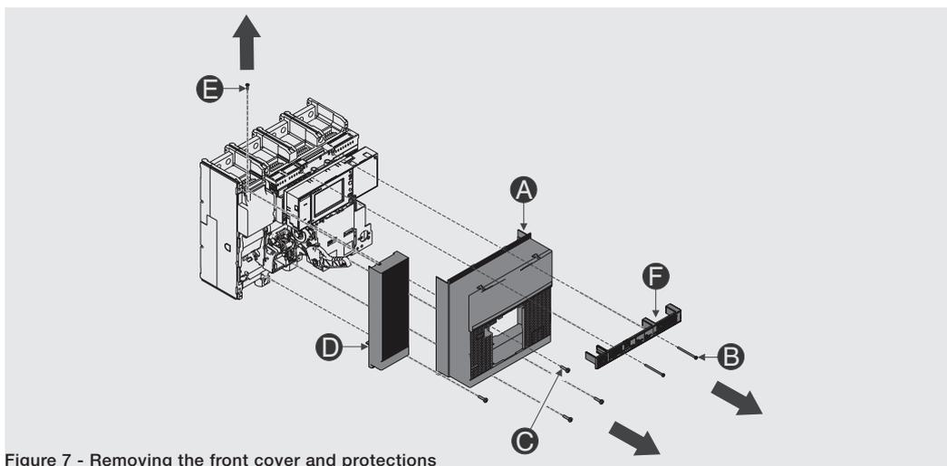
Figure 7 - Removing the front cover and protections
