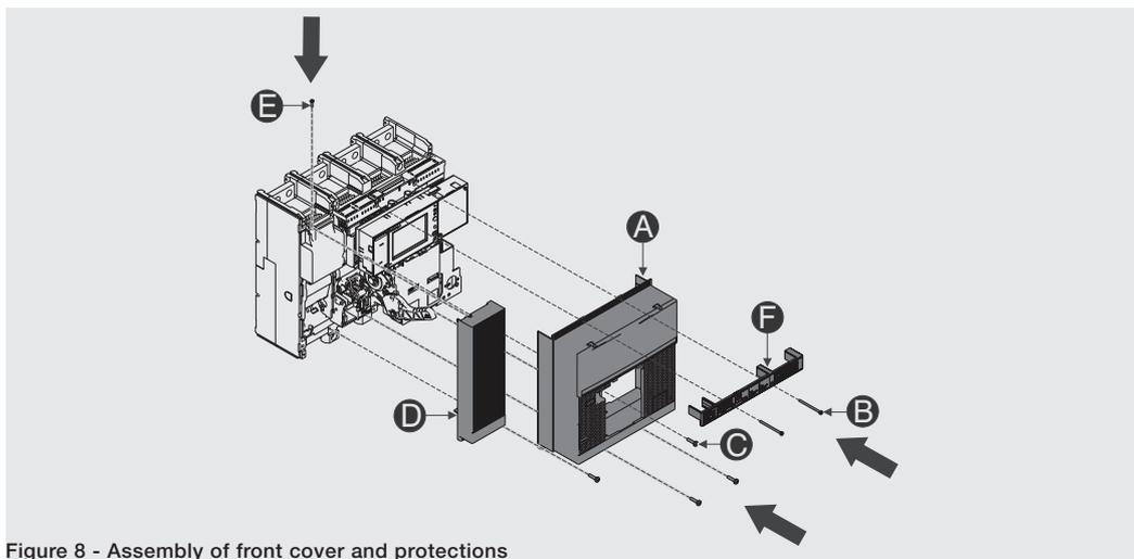
Figure 8 - Assembly of front cover and protections
