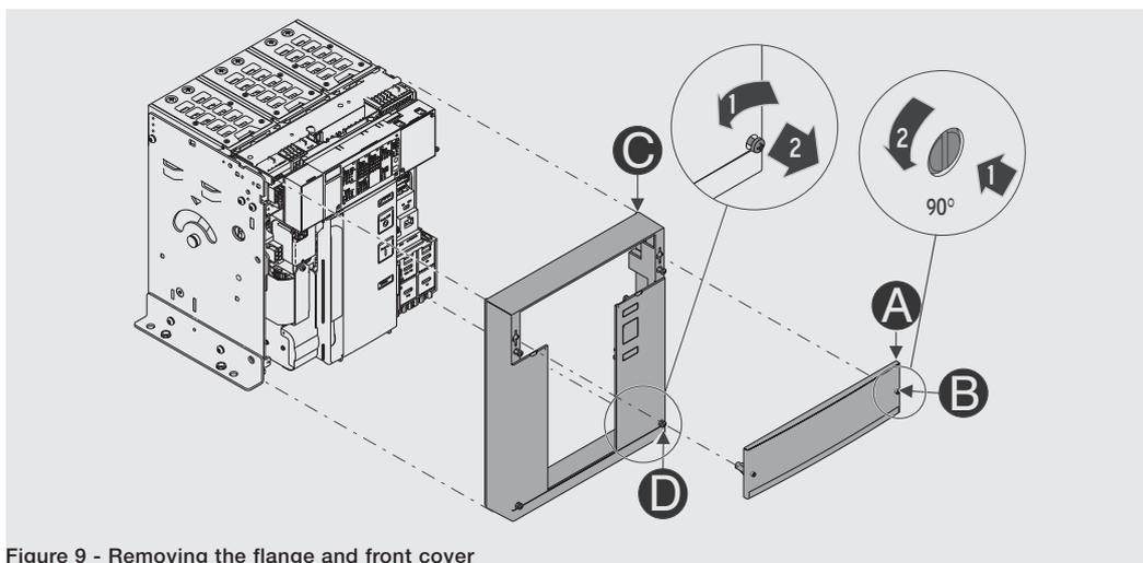
Figure 9 - Removing the flange and front cover
