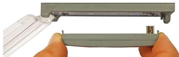
2. Plug the Ekip Display into the front of the ITS2.1.
