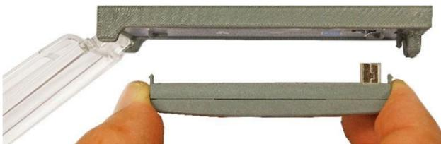
2. Plug in the Ekip Display carefully. Let the guide pin at the left side first slide into position. Then slide the right side into the USB plug in the ITS2.1.
