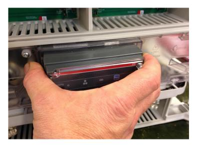
How to remove: Grab ITS2.1 or ITS2.D housing as shown and pull.
