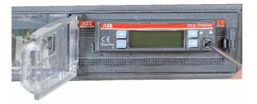
3. Fix the closing button by using a screw driver and rotate to closed position.
