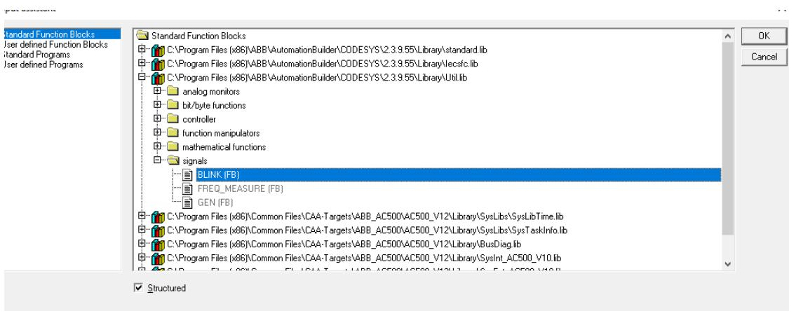
8. We continue create a function block “ETH\_MOD\_MAST” by CTRL+B and select Standard Function Blocks -> Ethernet\_AC500\_V10.lib -> MODBUS\_TCP-> ETH\_MOD\_MAST(FB) -> OK.
