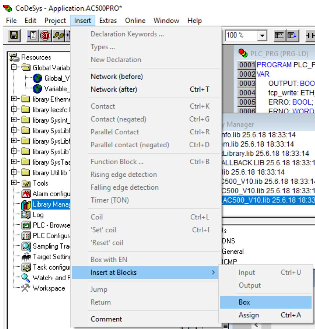
The default box is “AND”, and we insert “IP\_ADR\_STRING\_TO\_DWORD” at the blue marked area, then press ENTER. We can also find this box by pressing F2 when the marked area is selected. We insert IP-address in front of IP\_ADR of “IP\_ADR\_STRING\_TO\_DWORD”.
