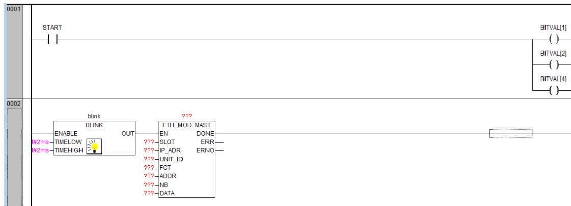
The **ETH\_MOD\_MAST** is a function block for sending/receiving OpenModbus on TCP/IP telegrams to/from an OpenModbus on TCP/IP Server. The function has inputs: EN, SLOT, IP\_ADDR, UNIT\_ID, FCT, ADDR, NB and DATA. Their definition is available from CoDeSys -> Resources -> Library Manager.
