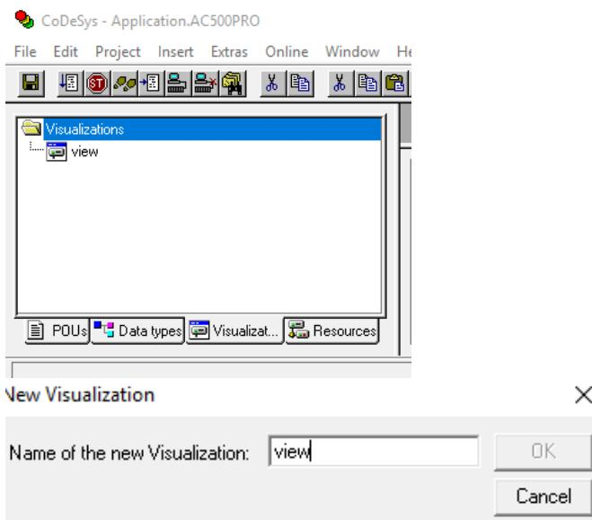
14. We draw a shape as the button
