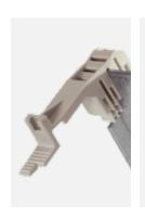
The fixing hooks and feet supplied in the standard versions are applied without having to use tools, making it possible to install the base plate at seven different depths inside the switchboard. They can also be adjusted at three further positions.
