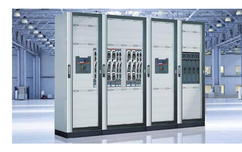
The ABB range of metal enclosures for main distribution has two fundamental elements with System pro E power Empty and 185 mm Busbar System. The columns have a functional height of 1800, 2100 mm and a functional depth of 300 and 500 mm. Five widths can be selected (functional from 250 mm to 1250 mm, with 250 mm steps) depending on the device type and quantity.
