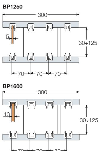
> Measurements are in millimetres
