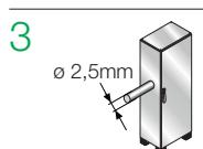
Protected against solid bodies with diameter or thickness greater than 2.5 mm
