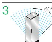
Protection against water droplets with enclosure at up to 60° from vertical
