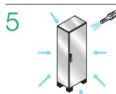
Protection against jets of water from all directions deployed through a nozzle
