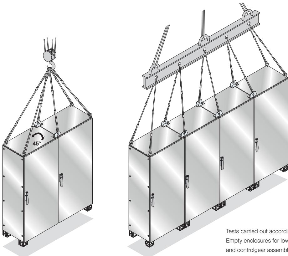
Tests carried out according to EN 62208 (par. 8.4) Standard
