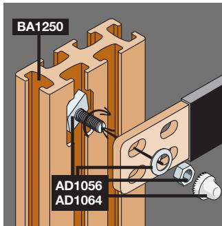
M8 self-locking hammer screw for fixing between conductors in any position along the busbar, guarantees a large contact surface.
