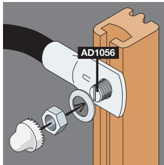
Direct branch by means of cable terminal for cross-section of cable up to 50mm<sup>2</sup>.
