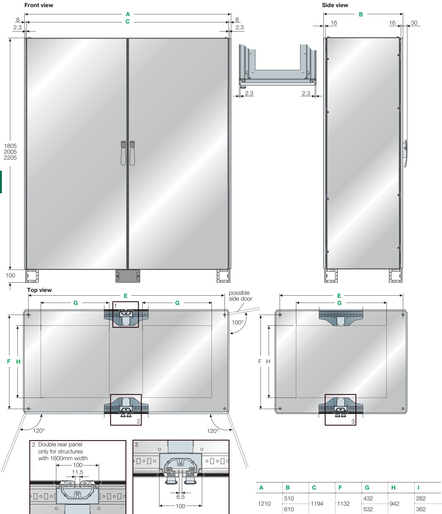
► Measurements are in millimetres
