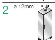
Protected against solid bodies with diameter greater than 12 mm or length greater than 80 mm
