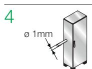
Protected against solid bodies with diameter or thickness greater than 1.0 mm
