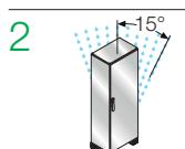
Protection against water droplets with enclosure at up to 15° from vertical
