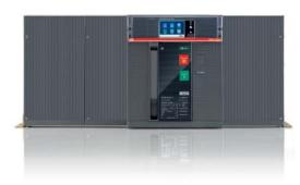
E1.2 offers 1200A with an interrupting rating up to 65kA at 508V and a short-time withstand rating of 50kA. It enables switchgear of 65kA to be built in widths of 16 inches, which are indispensable in places where reduced dimensions are essential, such as in naval and offshore installations.
