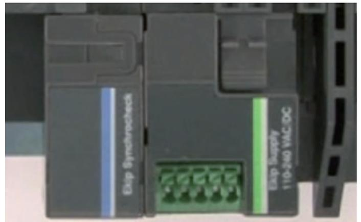
Figure 2 - Ekip Synchrocheck and Supply Modules installed in terminal box
