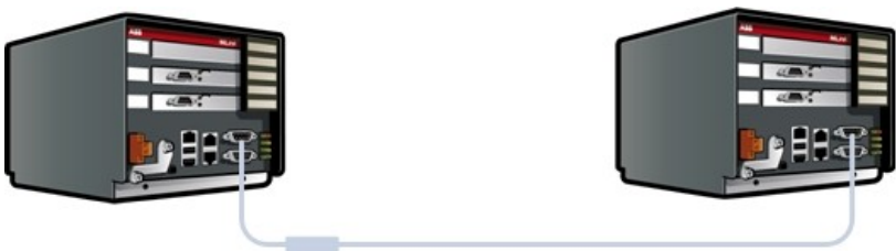
Figure 18 Serial 1 to serial 1 redundant link connections with ferrite core
