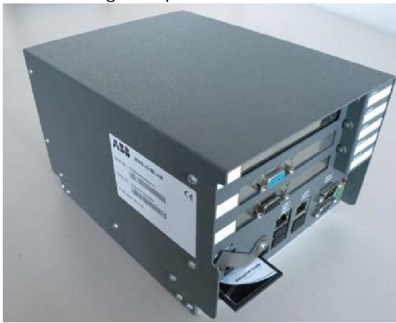
Figure 8 CF Card Insertion
