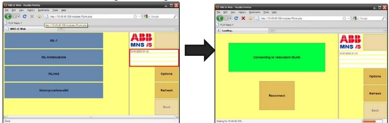
Figure 21 MView Redirecting to Redundant MNS Digital Gateway
