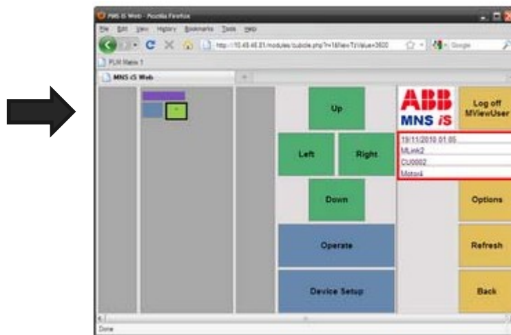
Figure 22 Redundancy error shown in MView by a red square
