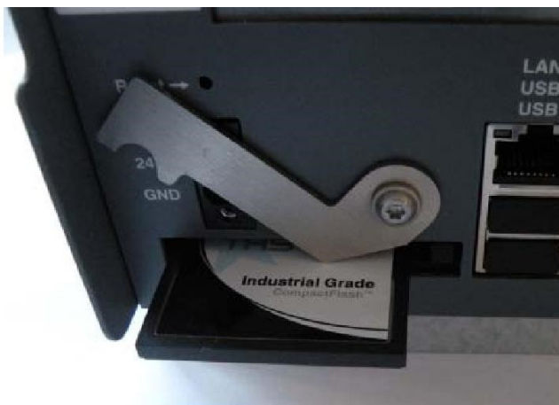
Figure 9 CF Card Insertion Detail
