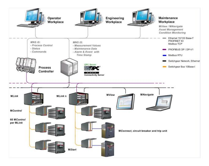
Fig. 3 System architecture with MConnect and Circuit breaker
