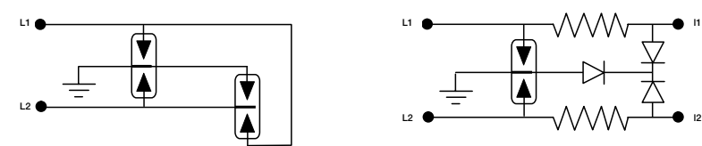
OVR TC 200 V in parallel OVR TC / xx V / 200 FR in series
