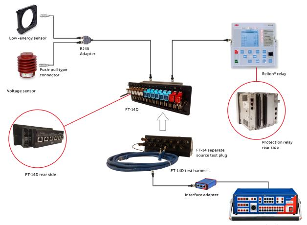
Protection relay test equipment
