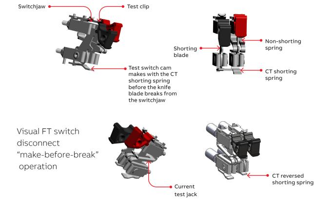
The reversed current shorting pole option positions the CT shorting spring, individual current jack and associated knife blades in reverse. The pole designations for this configuration are available only in sets of two and are described with two characters (C+C). The "+" sign is the indication for reversal. Current shorting is performed with the right hand blade versus the traditional left hand blade. Current monitoring is accessed with an individual current test jack in the left hand position.
