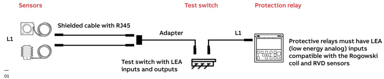
01 Minimized analog wiring in the switchgear increases reliability
