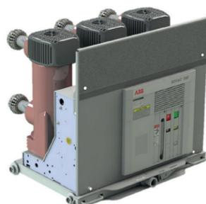
The ADVAC® G40 vacuum generator circuit breaker is available at 15 kV, 4000 A, 40 kA in compliance with IEEE/IEC 62271-37-013. The withdrawable ADVAC G40 offers a small footprint and full protection for power generation applications.
