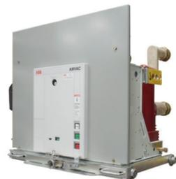
The AMVAC™ breaker is a magnetically actuated and latched breaker capable of a high number of operations due to its simplified design. Fully compliant with IEEE Standards C37.04, C37.06 and C37.09, the AMVAC breaker is a great fit when maintenance is a key concern.
