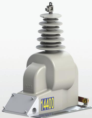
The VOG-15R is a lightweight voltage transformer with ResiVolt transient resistant technology, designed for use in line-to-ground metering and recloser applications.
