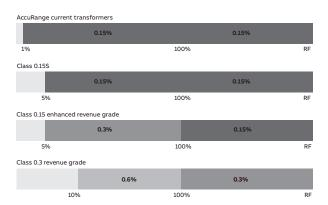
a great fit for variable load applications. Accuracy is guaranteed to be +/- 0.15% from 1% of nominal current through rating factor. ABB's extended range units deliver savings through improved accuracy metering and reduced inventory.
