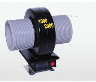
The LG-25-6513 and LGX-25-6513 outdoor current transformers are designed for use on substation structures where high current, large diameter primary conductors are used.
