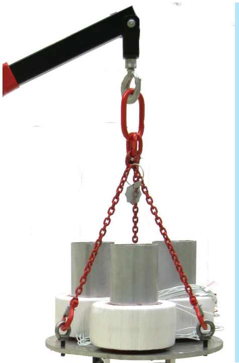
Fig. 2. Manipulation on crane with belts attached on 3 places
