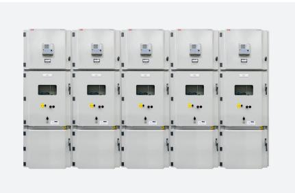
Each panel consists of two single units connected in double busbar arrangement. They can be equipped with circuit-breaker or contactor as well as with all the accessories available for the conventional units of the switchgear. Each panel is provided with a cubicle to take the auxiliary instrumentation, placed in the upper part.
