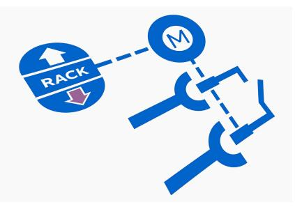
Truckmaster allows circuit breakers to be remotely racked in and out from a safe distance. The device can be simply and rapidly applied to the circuit breaker compartment door. Use of Truckmaster is the most effective way to ensure that operators work in total safety.
