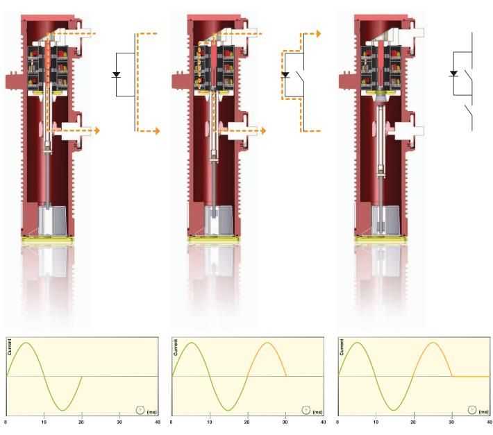
Switch in close position, capacitor bank is connected to the distribution network.
