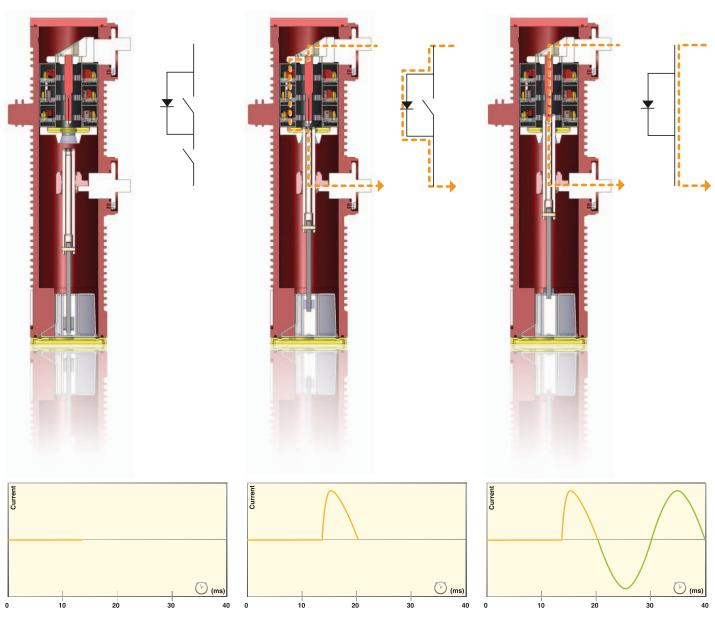
Switch in open position, capacitor bank is disconnected and isolated from the distribution network.
