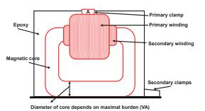
Single pole VT: connection is between phase and earth, e.g. 10 000 100 - v
