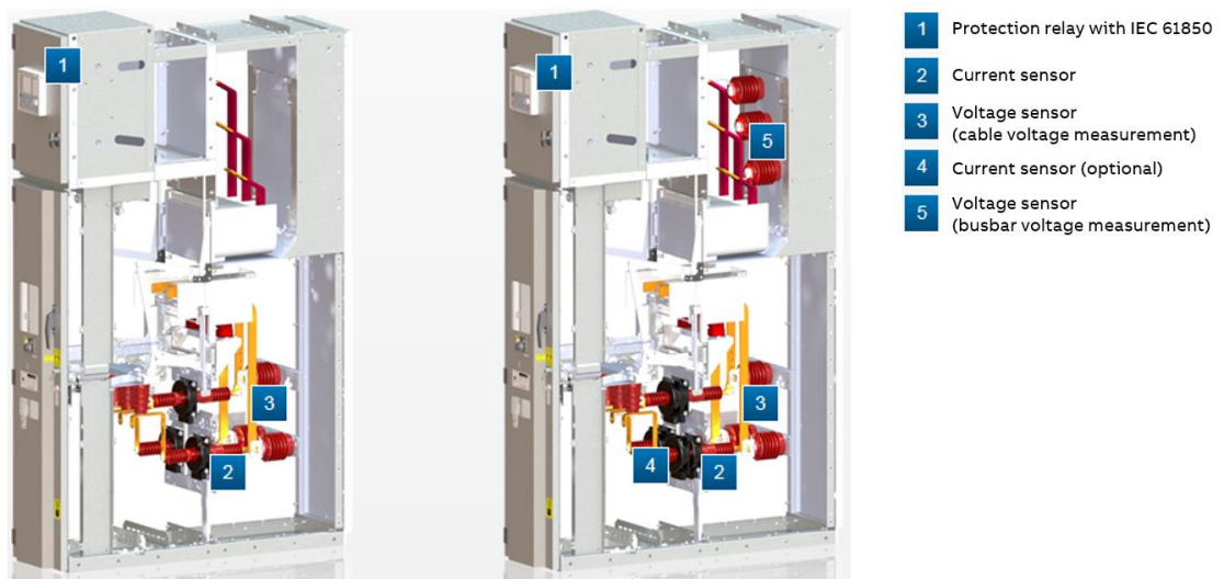
Figure 34: UniGear MCC Digital (12 kV, 400 A, 50 kA)
