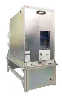
The comprehensive circuit breaker retrofitting solution integrates the earthing switch (ES) in the retrofill. This provides safety of operation by enabling earthing of the load side in the panels where ES is not present or it is not more reliable. The new earthing switch is fully interlocked with standard OneFit, providing renewal and highest reliability of all safety features. The optional CTs enable renewal of measurement and protection in one packaged and type tested solution.
