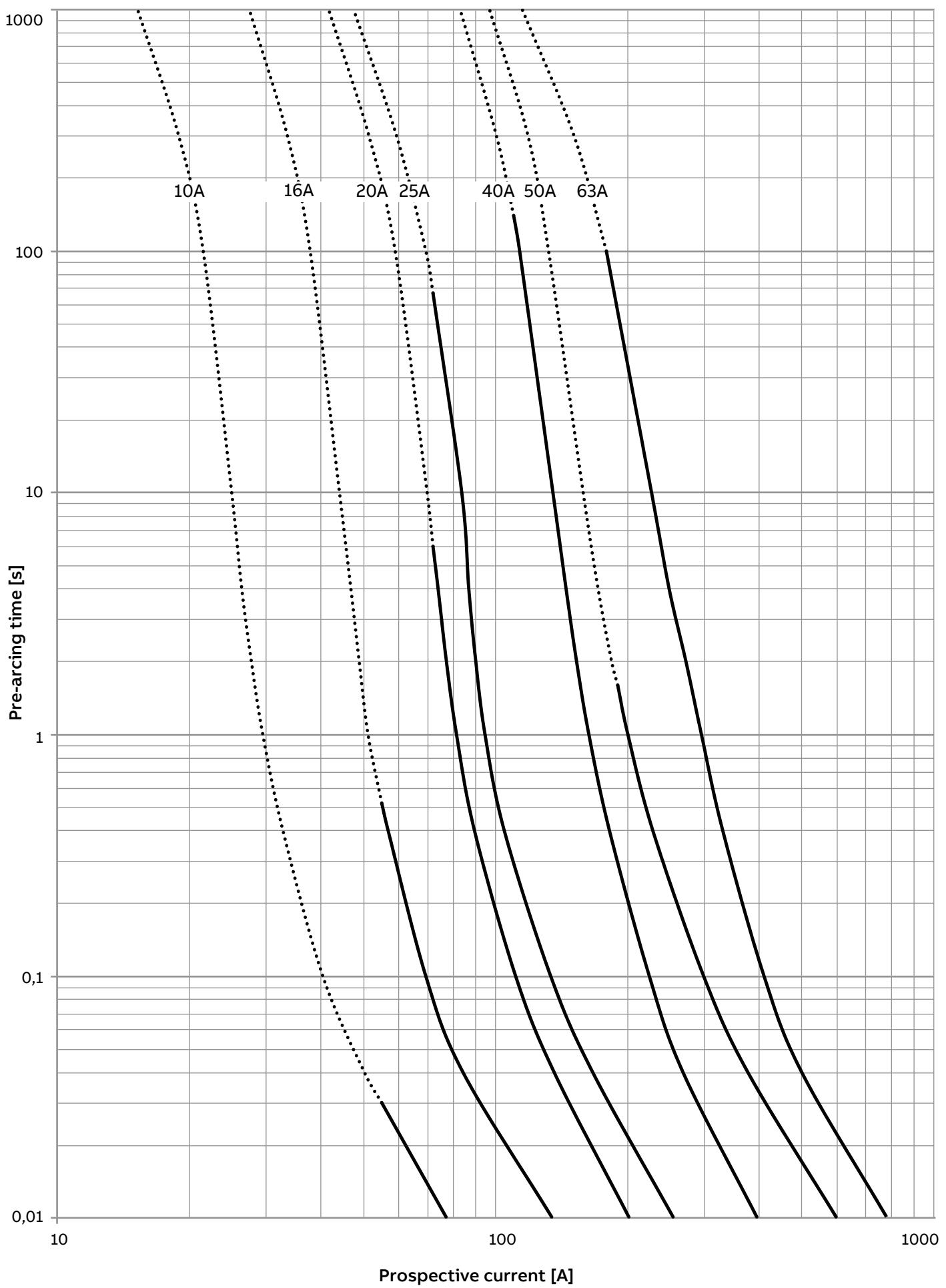
Characteristics show the average melting time as a function of the prospective current and are recorded from cold condition of fuse-link. The tolerance is  $\pm 10\%$  referred to the current.
