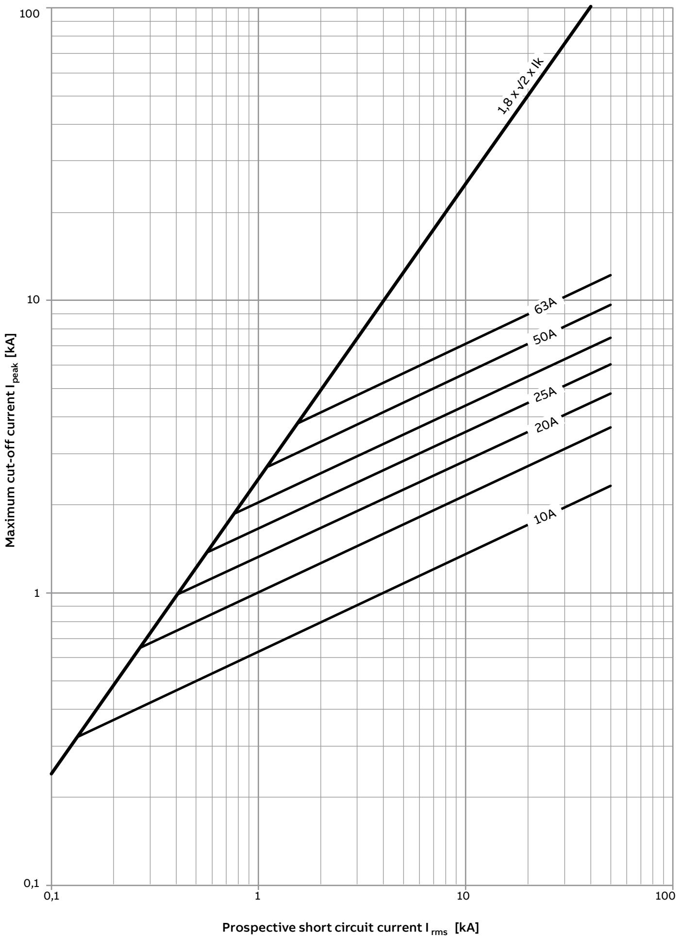
Characteristics show the cut-off current corresponding to a prospective short circuit current. Characteristics are valid for frequency 50Hz.
