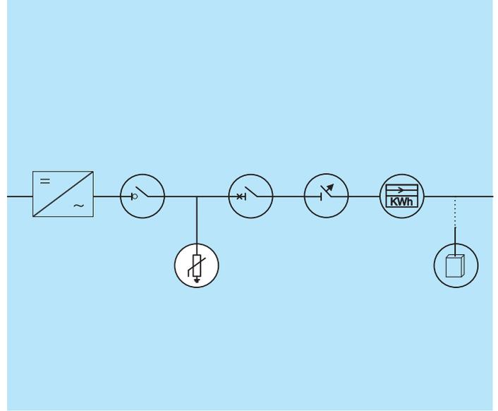
The OVR T2 protects inverters and installations from overvoltages and impulse currents, such as switching and lighting surges. The device ensures the limitation of overvoltage to an acceptable level for the equipment to be protected.
