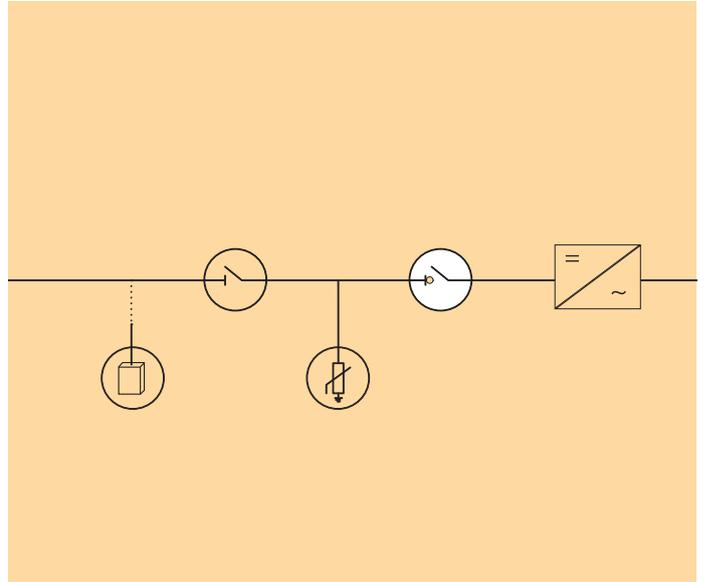
The switch disconnecter is used as a main switch for PV systems – the whole DC side can be safely isolated, either locally or remotely. The device offers safety-relevant isolation properties.
