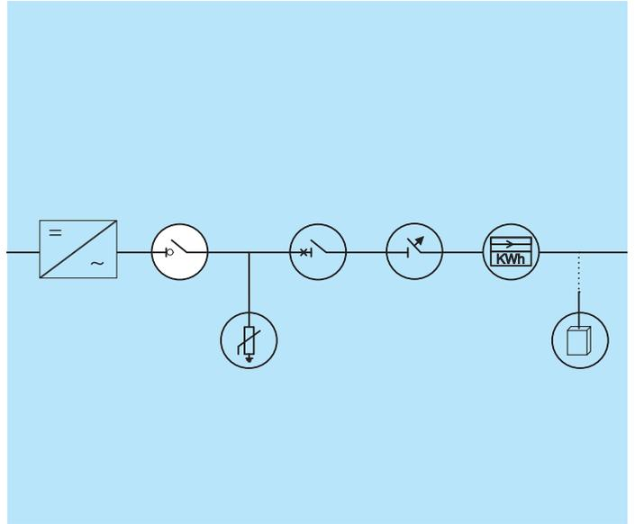
The isolator is used as a master switch on the AC side. It offers reliable and safe switching under loads.
