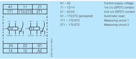
Connection diagram CM-MSS.51
