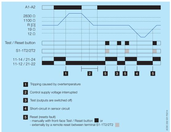
Manual or remote reset (= non-volatile fault storage)
