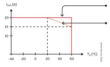
Normal application (up to 50 % buffer mode, 5 charging and discharging cycles in direct series)
