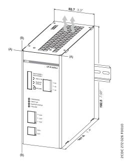
The device has to be mounted horizontally with the input terminals on the bottom. In order to ensure a sufficient convection, the minimum distance to the other modules must be not less than 80 mm (3.15 in) in vertical direction. Minimum distance in horizontal direction is not necessary.
