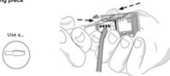
5.2 Pry upwards to release the upper hook.
