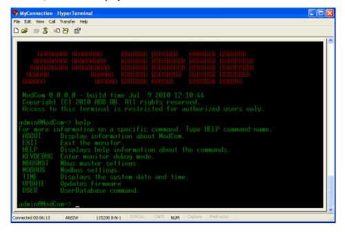
To find out more about a specific command, type help and the name of the command, i.e., help modbus.
