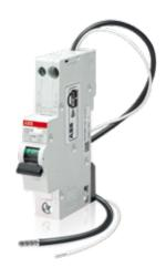
The 1P+N electronic residual current circuit-breakers with overcurrent protection (RCBOs) DSE201 meet the demand for devices that fully protect modern installations against short-circuit currents, overloads earth fault currents and indirect contacts, providing additional protection against direct contacts (30 mA versions). Each RCBO is fitted with a functional earth wire to guarantee the highest level of safety, even in case of loss of neutral.
