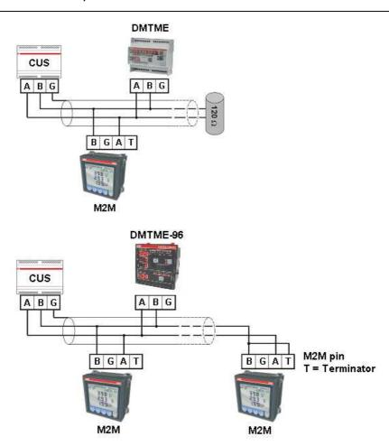
In the previous figure, if the M2M is the last instrument installed in the RS485 network, is possibile to avoid the terminal resistor connecting pin T with pin B.
