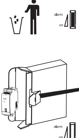
Internal protection of the device will disconnect the surge protective components at the end of their useful life, but will maintain power to the load, therefore left unprotected. If this situation is not desirable for the installation, replace the plug according to the instructions in the present document.
