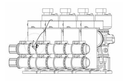
The portable emergency pump for operating mechanisms allows a manual charging of the circuit breaker operating mechanism - especially when the power supply has failed temporarily or when the oil pump of the operating mechanism has any malfunction. Through this manual operation, the energy storage can be charged until a safe OPEN operation is possible.
