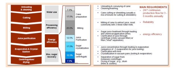
Figure 6: Energy consumption highlights in sugar production
