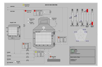
Figure 5: This graphical interface for the vacuum batch pan library enables the operator to increase the operational efficiency while decreasing the operations error
