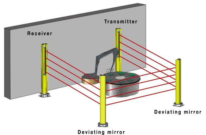
Perimeter protection with two Orion1 Mirrors in Orion Stands.
