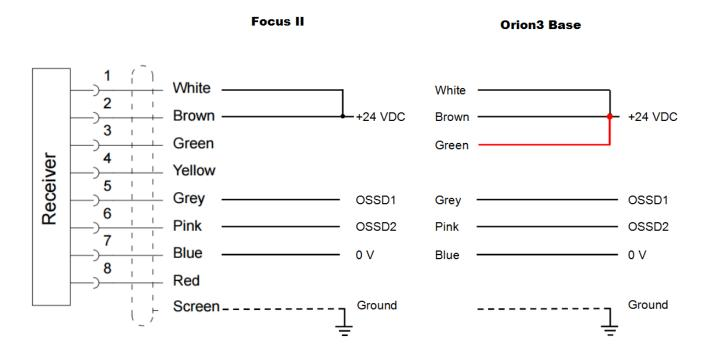
Reset button connected to the light curtain, no EDM\*
