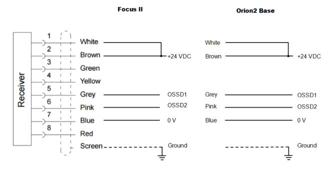
Reset button connected to the light curtain, no EDM\*
