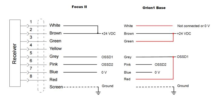
Reset button connected to the light curtain, no EDM\*
