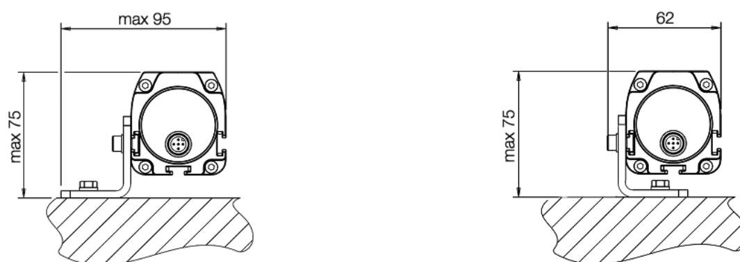
Figure 36 – Dimensions of the angled fixing bracket with a profile
