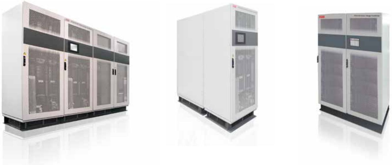
The PCS100 AVC range offered by ABB corrects voltage sags and surges within a few milliseconds, and is available in load capacities of 150 kVA to 2.4 MVA
