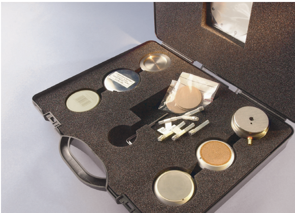
Accessories such as check nozzles, extra backings, vaseline and zero film are supplied in an accessory case.
