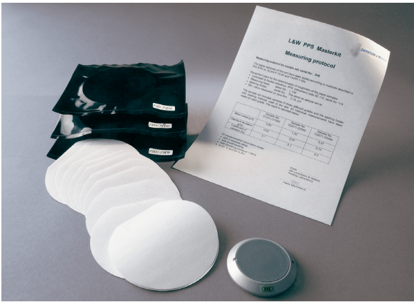
L&W PPS Master Kit contains three different paper samples with set points for PPS surface roughness. A soft backing is also included.
