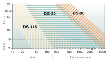
L&W Moisture Sensor DS-115 covers all paper grades from fine paper to paperboard. For pulp or very heavy paperboard, we provide the well proven moisture sensors; L&W Moisture Sensors DS-20 and DS-30.
