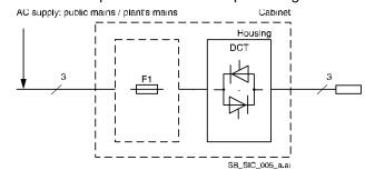
The figure shows the arrangement of external fuses in the thyristor power controller.
