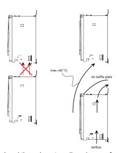
Lead the exhaust cooling air away from the unit above. Distances table above.
